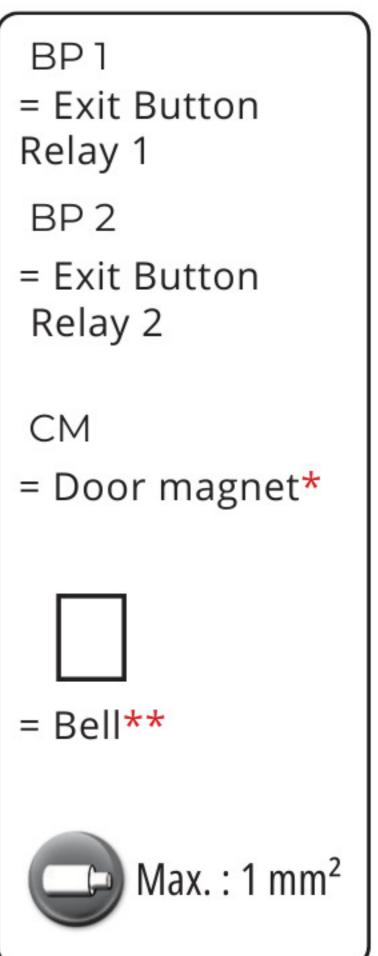
\*Door magnet = Detection of door status. When someone opens the door and comes in, the door is closed. The system will automatically detect the door status and lock the door, even though there is still a delay period.
