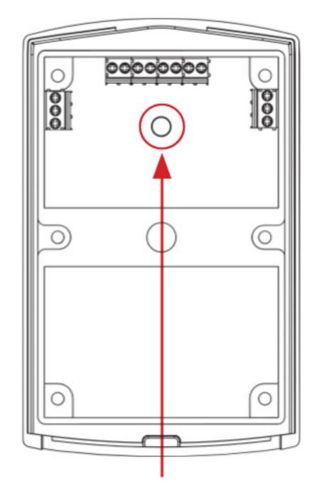
Anti-tamper photocell. To activate the function, please refer to page 20/20 «Enable / Disable the tamper function»
